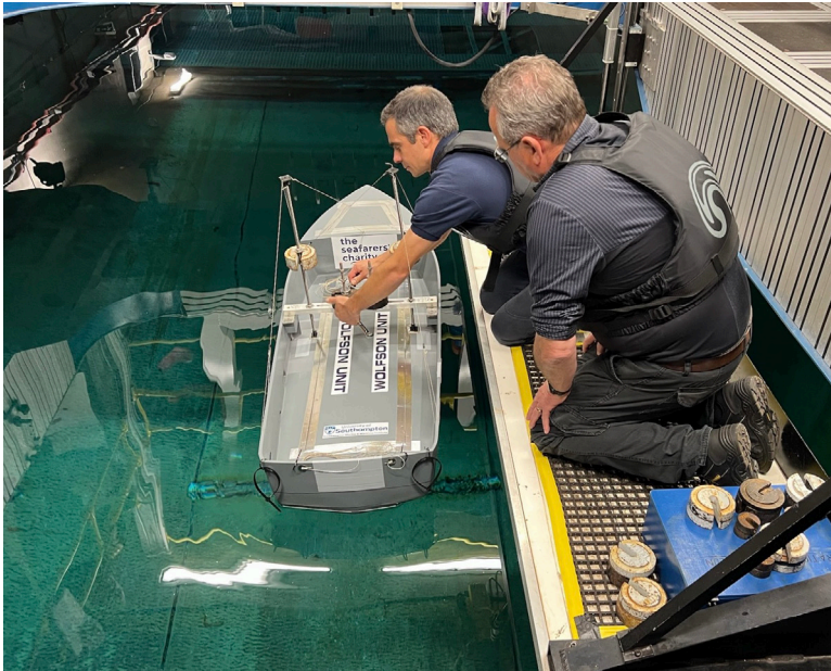
▲ Matteo Scarponi adjusts the loading of the monohull model, watched by Iain MacAulay of the Western Isles Fishermen's Association.
