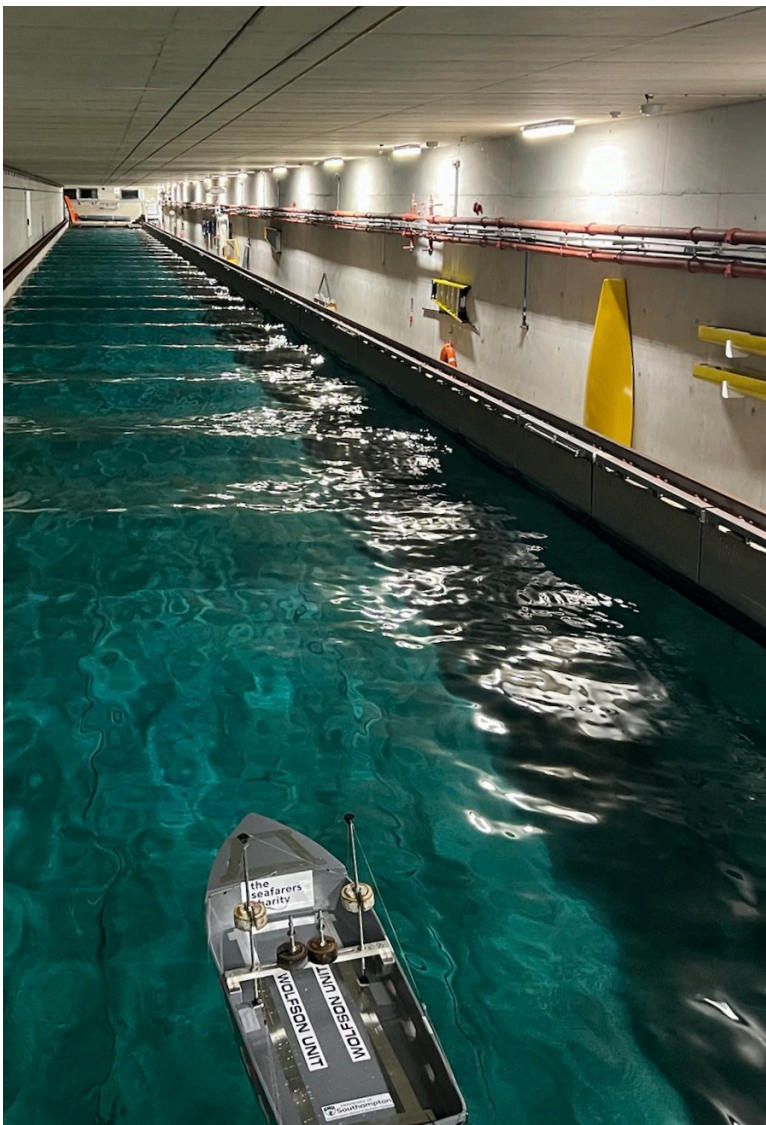
▲ A series of tests in Southampton University's 138m Boldrewood Towing Tank allowed a number of the provisions of the MCA code of practice to be explored under different load conditions and in varying sea states.
