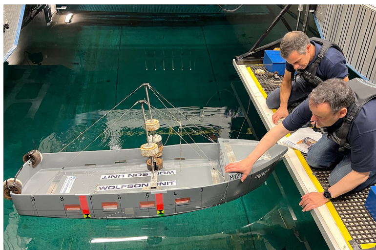
▲ Dr Matteo Scarponi, principal consulting engineer at the Wolfson Unit (left), with David Grant of UHI Shetland, sighting the Wolfson freeboard mark on the topsides of the monohull scale model.
