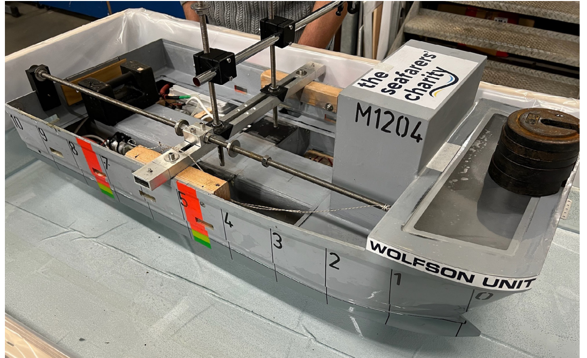
▲ Weights on the scale model allowed fine adjustments to be made to simulate different load conditions.
