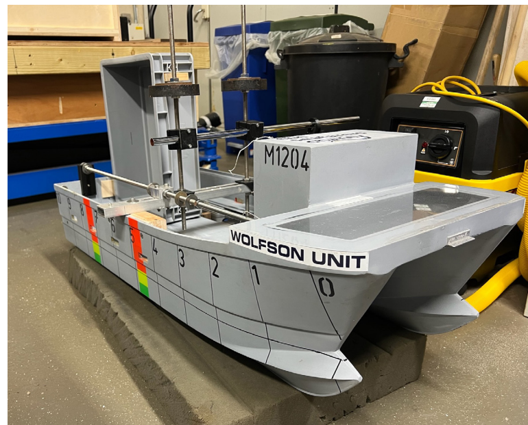
▲ The second phase of testing focused on a scale model of a 9m hard chine catamaran, following input from the NFFO. (Photos: Seafish)
